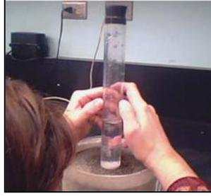
Figure 2. Testing one sample with infiltrometer.
