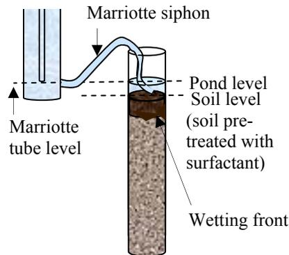
Figure 1. The key elements in the infiltration rate experimental setup.
