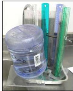
Figure 3. Four replicates undergoing treatment in the capillary rise experiment.
