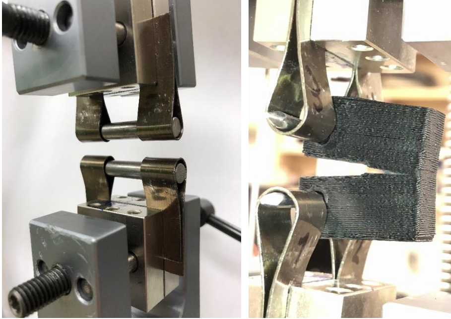
Figure 6.2: Compact tension sample holding set-up for fracture tests
