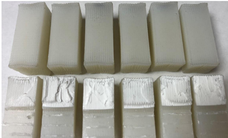
Figure 6.4: Fracture- and top-surfaces of pure ABS samples with 10 mm thickness
