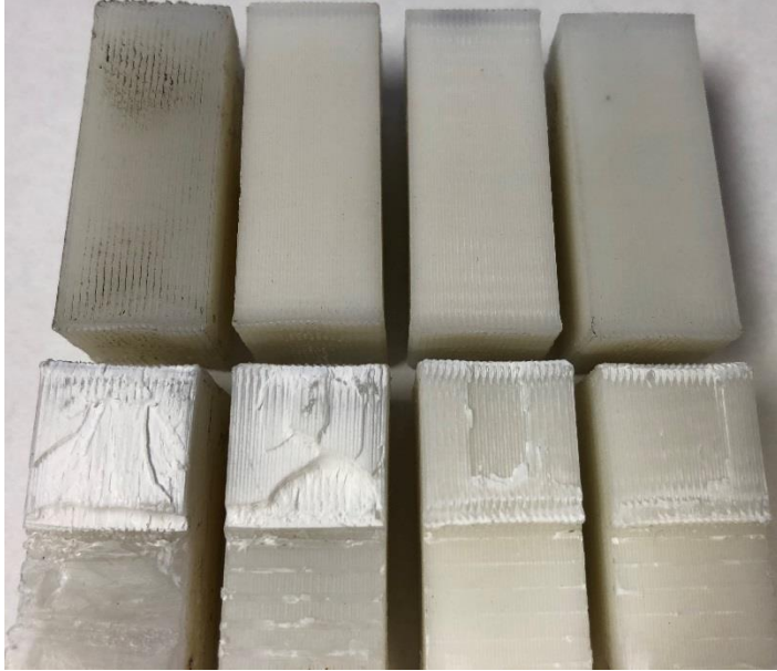
Figure 6.3: Fracture- and top-surfaces of pure ABS samples with 15 mm thickness
