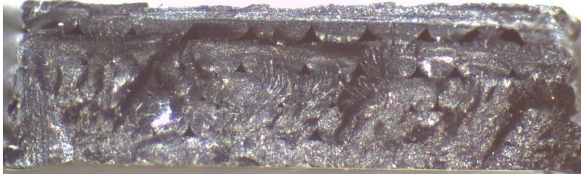
Figure 4.6: Fracture surface of a sample printed with 0.5 mm nozzle diameter and 0.35 mm line width
