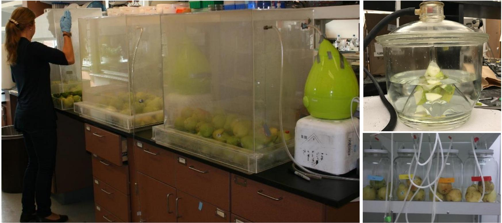
**Figure 3.18** Left: Ultrasonic humidification chamber set up for ripening compound and control solution administration.
